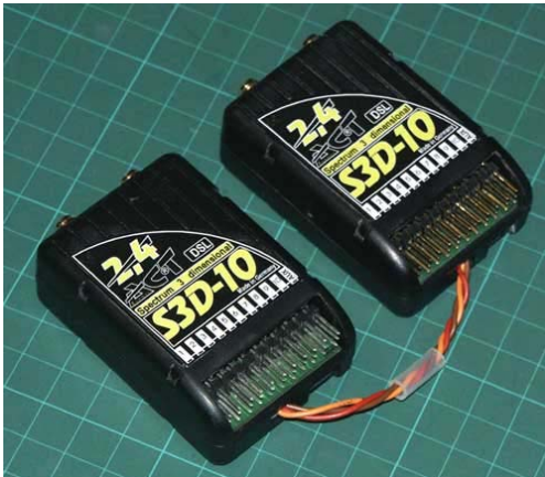
Dual-3D-Diversity use by connecting two S3D receivers
