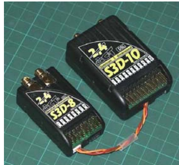
Dual-3D-Diversity use by connecting two S3D receivers
