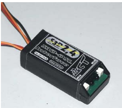
S3D-DSL-Converter, for use of 35MHz + 2,4GHz-receivers simultaneously
